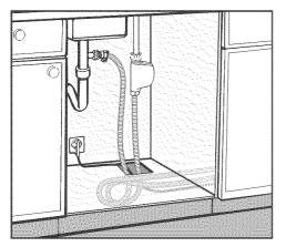
Make a 2" x 4" (5 x 10 cm) cut out in the side or bottom of the cabinet adjoining the dishwasher. This cut out is necessary for connections to pass through. Make certain that there are no rough edges that could damage the power cord or hoses. If metal cabinets are used, place the supplied rubber grommet around the edge of the opening before passing the cable through.
